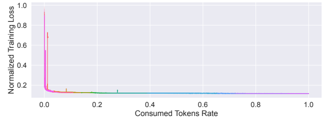
Figure 20. The normalized training loss curve of a real production job on more than 10,000 GPUs for months, training a MoE model with 20B activated and 200B total parameters on multi-trillion tokens. Different colors indicate training restarts.
